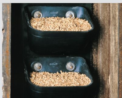
Buckets fitted to a belt conveying fodder.
