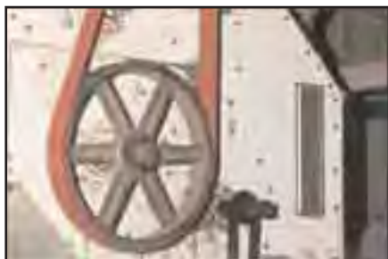
Cotton Cleaner: 4 x "B" section— Can replace damaged sections following jamming and stalling of drive.
