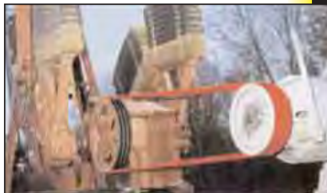
Oil Pumping Unit: 3 x "C" section—Handles shock loads, resists dry rotting and provides on-site availability.
