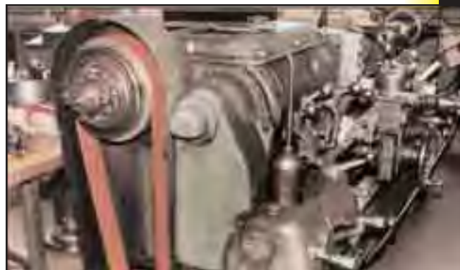
Lathe: 4 x "B" section—Oil and heat resistance plus reduced transmitted vibration to spindle.
